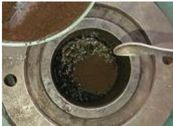
Step 5 Pour the mixture into the mold and press it by hand
