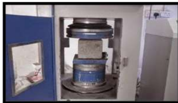
Fig.3. Setup for Compressive Strength Test
