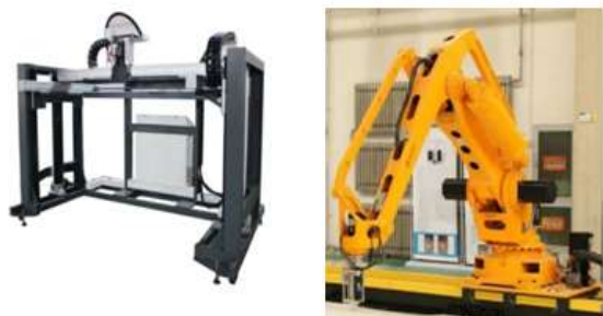
Figure 3: Some commercial 3D concrete printers.
