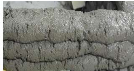
Figure 7: The print is slightly cracked
