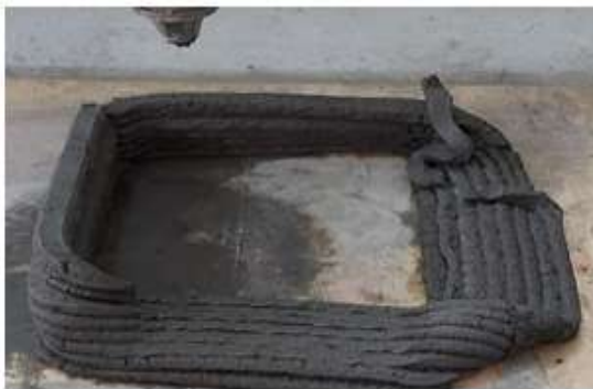
Figure 9: Pour pattern due to geometric deviation between layer 1 and layer 2
