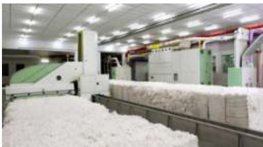
Figure 1: Automatic bale opening and mixing
