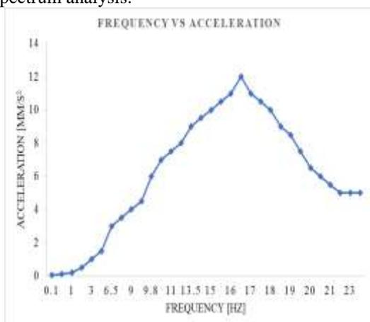
Figure 10 Acceleration vs frequency
