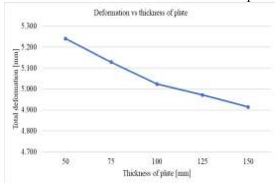
Figure 13 Total deformation vs thickness of plate
