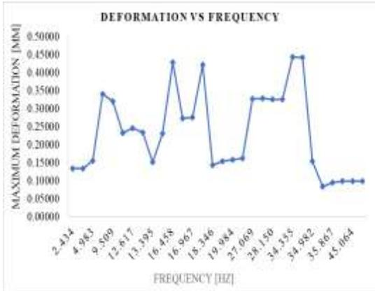
Figure 9 Frequency vs deformation for 30modes
