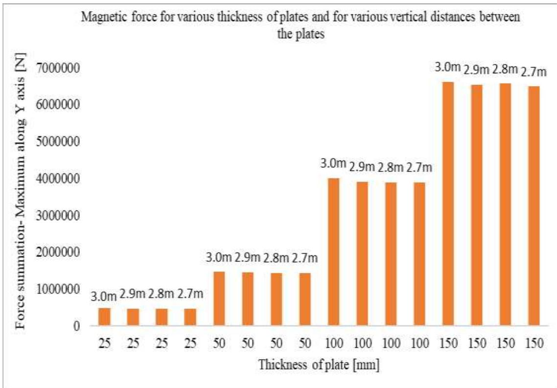
Figure 19 Magnetic summation force for various thickness of plates and for various vertical distances
