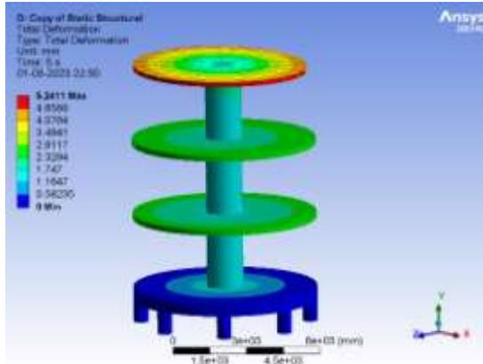
The figure 5 shows that the maximum deformation caused at the end of the cantilever slab is 5.2411mm.
