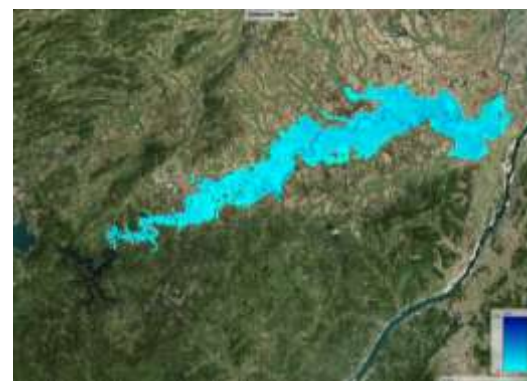
Dam failure 24 h
