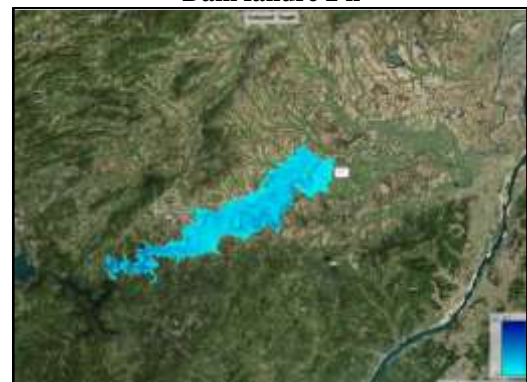
Dam failure 10 h
