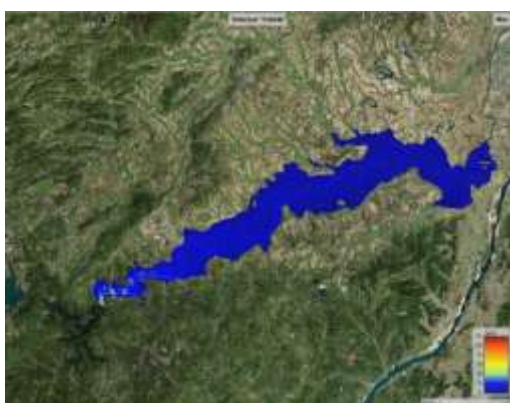
Figure 5 Maximum flow velocity distribution
