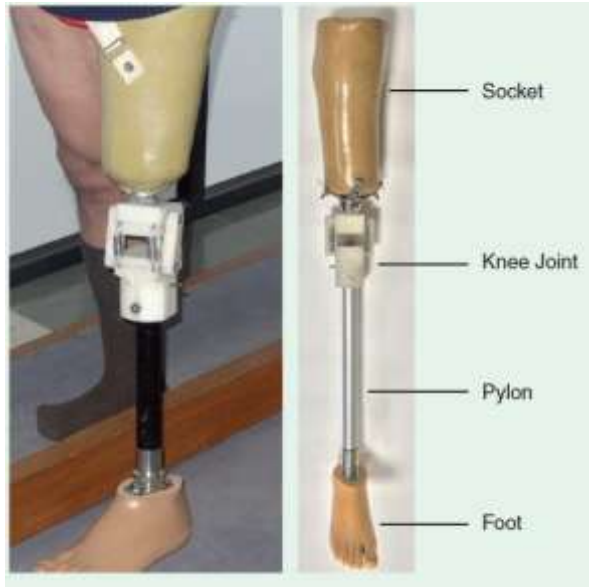
Figure 1. The various parts of a lower-limb prosthesis. [8]
