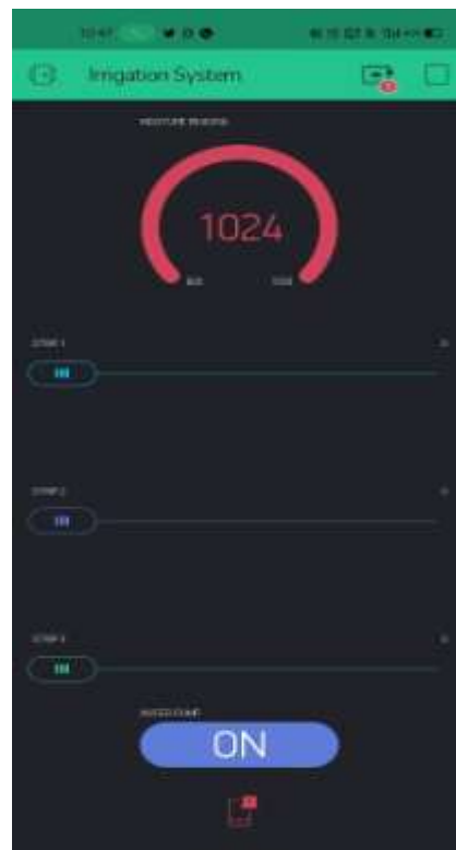
Fig. 6. Live readings when the irrigation pump is in the "ON" state.
