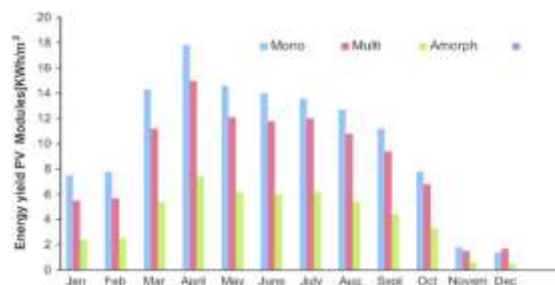
Fig-7: The graph shows a comparison in efficiency of the three cells
