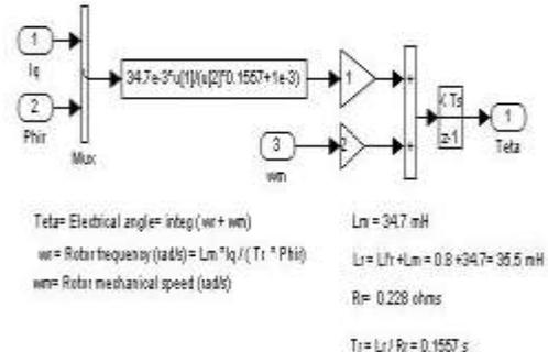
Fig 3.4: Theta Calculation block
