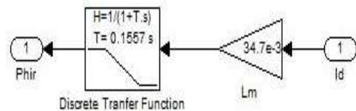
Fig. 3.3: Flux Calculation Block
