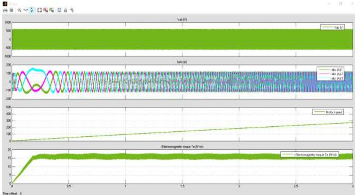
**Fig 4.1:** The graph shows the Voltage generated out from the inverter. Fig 4.2.2 shows the current output, fig 4.2.3 shows the speed of the motor. Fig 4.2.4 shows the torque which keeps changing itself to stabilize the motor at the higher speed it is controlled by the FUZZY LOGIC Controller.
