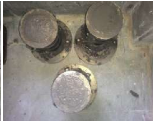
Figure3.7: Casting of Cylinder Specimen
