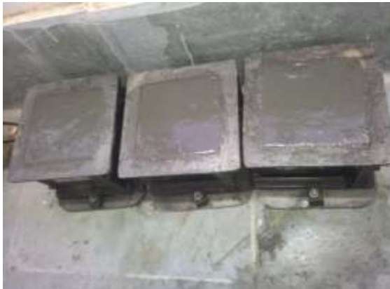
Figure3.6: Casting of Cube Specimen
