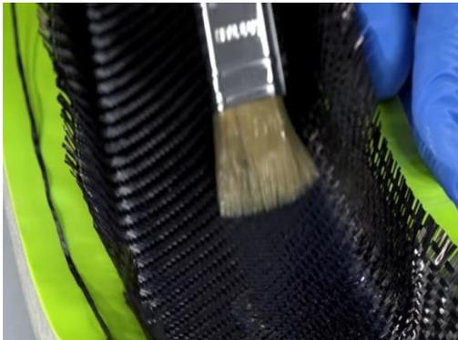
**Figure 7:** Lamination of the Part.
