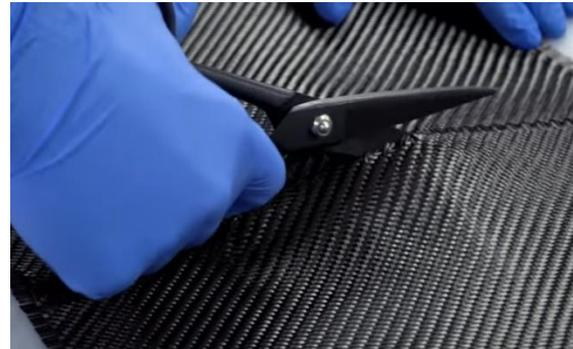
**Figure 4:** Cutting reinforcement of carbon fiber cloth
