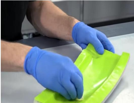
**Figure 2:** Application of mold release wax to the mold
