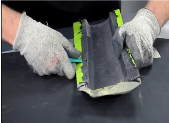
**Figure 9:** Demoulding of the cured part.
