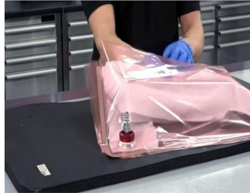
**Figure 8:** Vacuum bagging of the part.
