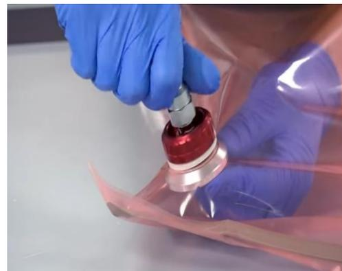
**Figure 5:** Preparation of the vacuum bag.
