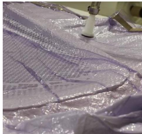
Figure 1: Vacuum Bagging Process
