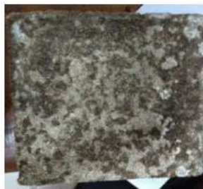
Fig 3. Particle board from Water hyacinth, 60:40 ratio
