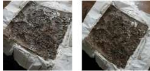
Fig 4. Particle board from Water hyacinth, 70:30 ratio
