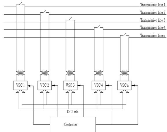
The IPFC provides several operation functions depending on the system operating requirements, such as independent active and reactive power flow control, transmission angle regulation and transmission line impedance control.
