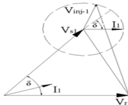
phasor operating area is a circle and depends on its amplitude and angle, so the voltage drop across the transmission line can be regulated.
