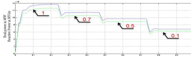
Fig. 6.12: Real and Reactive power flow on line 2 for the variation of the  $MI_2$
