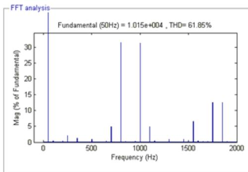
Fig. 6.4a: Harmonic analysis for line voltage
