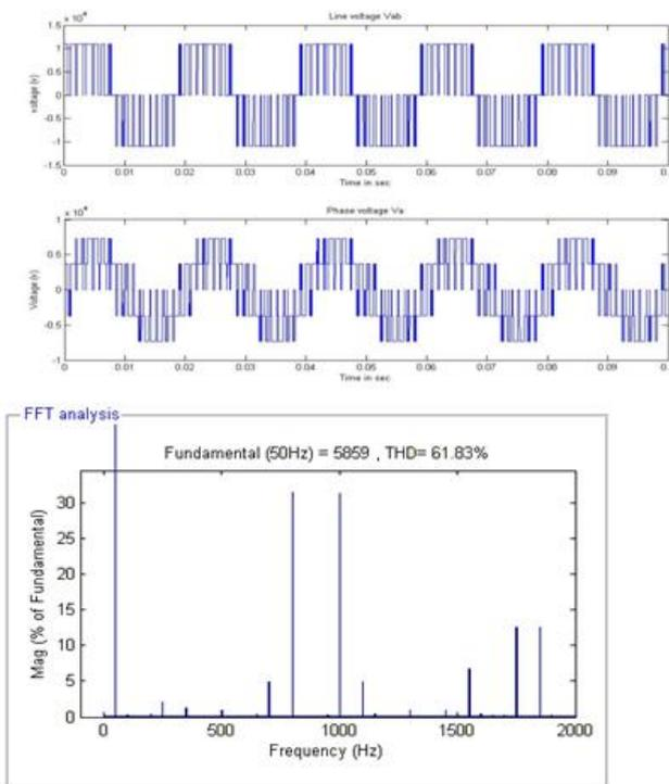
Fig. 6.3a: Inverter output line voltage
