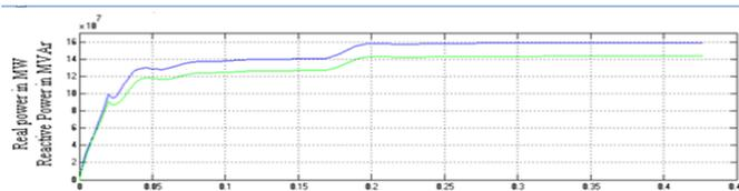
Fig. 6.14: Real and Reactive power flow on line 2 for the variation of the  $MI_2$
