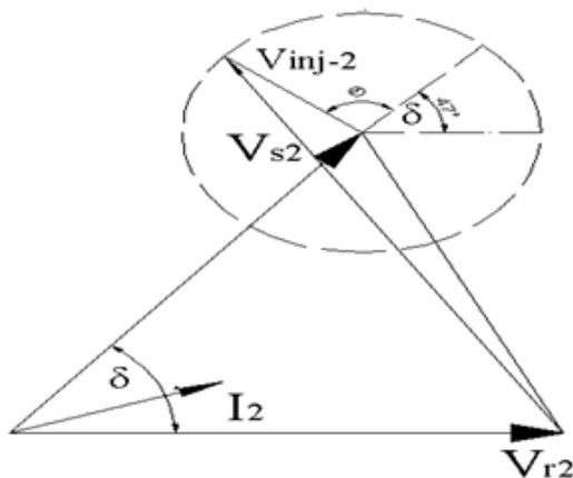
If  $|S_0| = 1.0$  and  $X/R = 10$ , then the radius of the circle is 5.025 Pu. Fig. 3.5 shows the control characteristics for  $P_0 = 1.0$ ,  $Q_0 = 0.0$ , with  $|S_0| = 1.0$ . The range of operation of a SSSC is only a part of the circle around the operating point  $S_0$ . This is due to the limitations imposed by the rating of SSSC. Fig. 3.5 also shows the range of operation of a SSSC which is bounded by a circle with  $S_0$  as centre and radius =  $|V_{Cmax}| V / Z$
