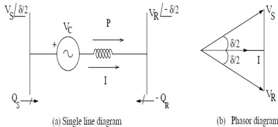
Fig.: Single line diagram of SSSC, Fig. 3.3(a):
