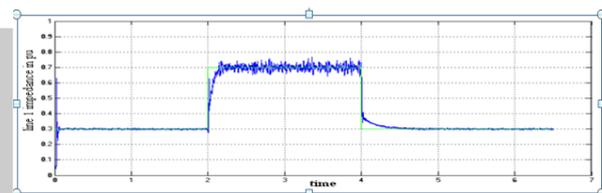
Fig. 6.18: Step change in injected impedance from 0.3pu to 0.7pu
