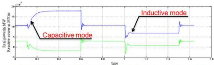
Fig. 6.9: Variation of Real & Reactive power supplied by the source for different mode
