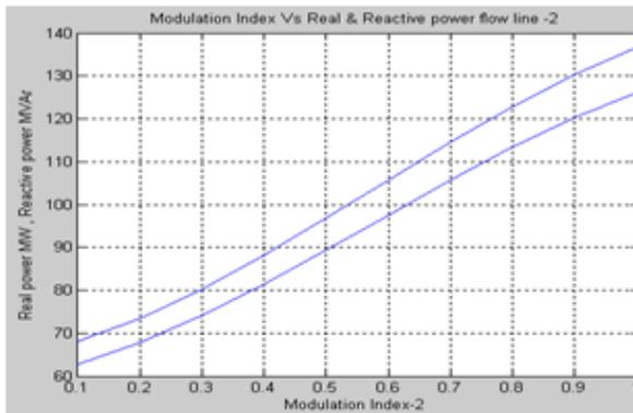
Fig. 6.16: Modulation index Vs P&Q on line 2
