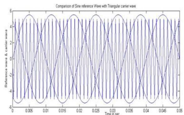
Fig. 6.1: SPWM Switching Waveforms
