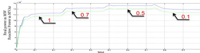
Fig. 6.13: Real and Reactive power flow on line 1 for the variation of the  $MI_2$
