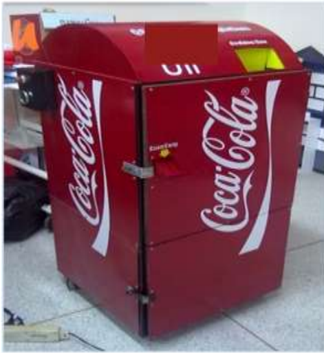
Fig 1.6 Image showing the external structure of the can receiver.
