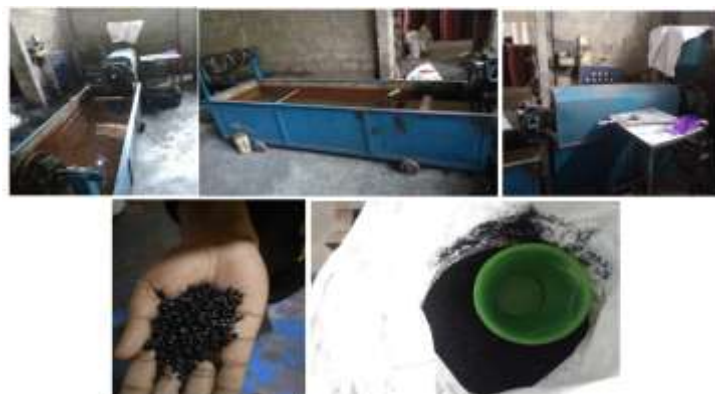
a)cooling tank fixed near the plastic mixer machine b)cooling tank c)Plastic Mixer Machine d)Granules finally obtained
