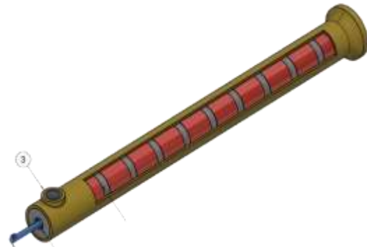
Figure 14: External Heater Bands with Fibreglass Insulation Wrap (Quarter-sectioned)
