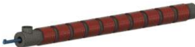
Figure 19: Meshed Scenario 1- Exposed Heater Bands
