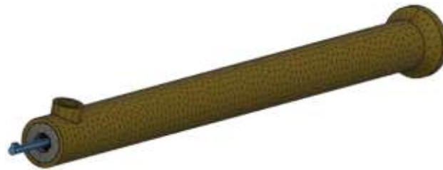
Figure 20: Meshed Scenario 2 Fibreglass Insulation Wrap
