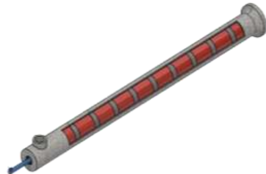
Figure 15: External Heater Bands with Composite Shell (Quarter-sectioned)
