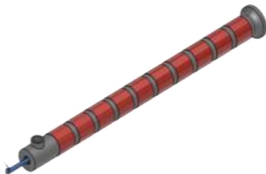
Figure 13: External Heater Bands with No Insulation
