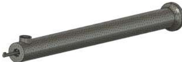
Figure 21: Meshed Scenario 3- Composite Shell Enclosure
