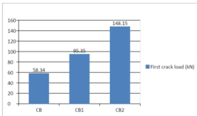
**Graph 4.2. Comparison of first crack load (12% fiber volume)**
