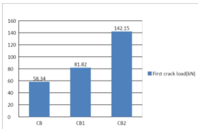
**Graph 4.1. Comparison of first crack load (10% fiber volume)**
