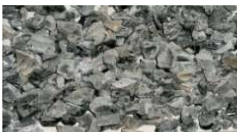
Figure No.2.2: Plastic waste after Shredding and cutting
