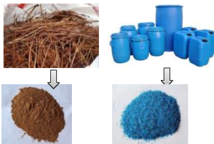
Fig.1 Raw materials and its powdered form (Pine needle and HDPE)
