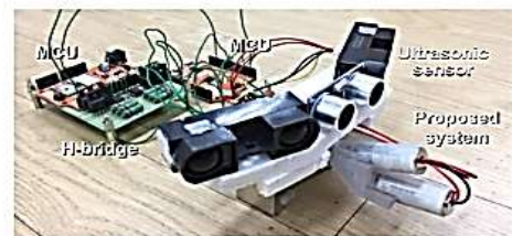
Fig. 23. Implementation of the proposed on-road projection with an ultrasonic sensor.
