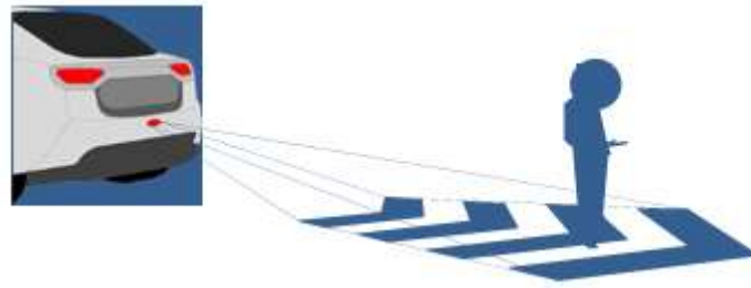
Fig. 1. Conventional vehicle warning system using on-road short-range projection with a static pattern.
