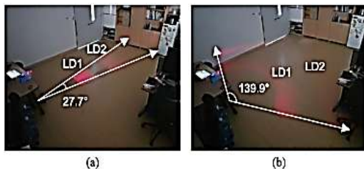
Fig. 22. Projection angle control for LD1 and LD2. (a) Narrow and (b) wide.
