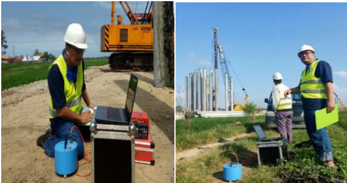
Figure 1. Measurement Of The Level Of Vibration At A Distance Of 10m And 70m
