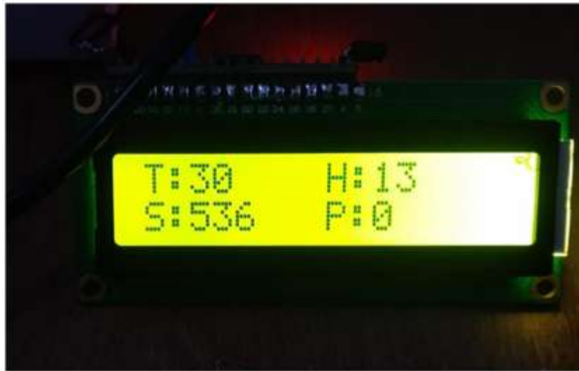
Fig 4.5: Smoke is sensed and detected more than 350
