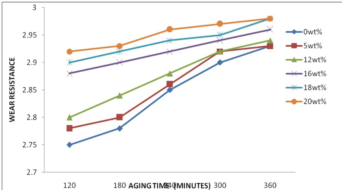
**Chart-2:** Effect of aging time on the wear resistance of Al-Si-Fe reinforced with varying percentage of CSA at 250°C.
