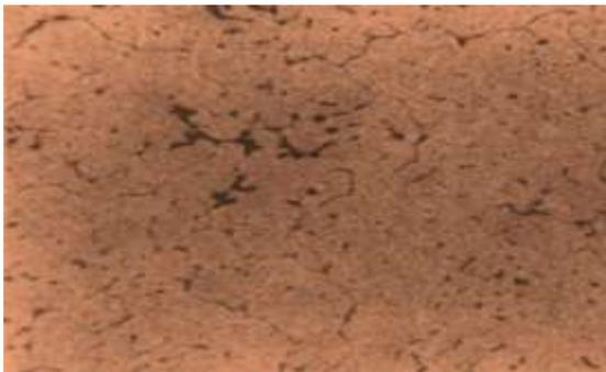
Plate 4.1: Microstructure of Al-Si-Fe matrix
