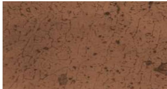
Plate 4.2: Microstructure of 18wt% of CSA reinforced Al-Si-Fe composite at 95 °C and at a holding time of 120 mins.
